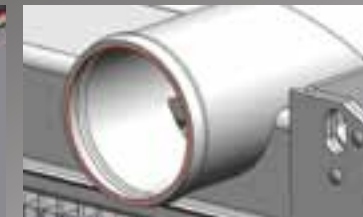
Increased connection wall thickness by 42%
