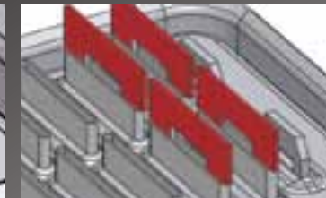
Tube reinforcement inserts
