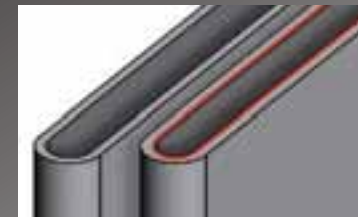
Increased Tube's wall thickness by 35%
