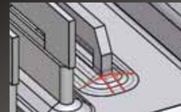
Low-profile embosses around the side-plate slots
