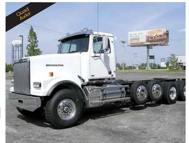
2012 WESTERN STAR 4900FA Det. DD13, 450 HP, Eng. Brake, 8LL, Chalmers Susp. 4.11 Ratio, 252" WB, 22.5 Tires, Alum. Wheels, Quad Axle, 20 # FA, 40 # RA, 2-13,200# Steerable pushers, full lockers, 162" CT, Stk #: 143677
