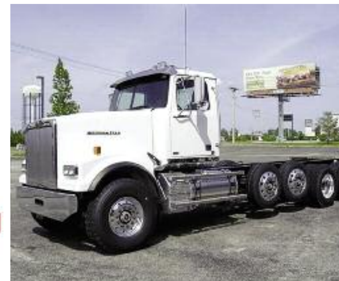
2012 WESTERN STAR 4900FA Det. DD13, 450 HP, Eng. Brake, 8LL, Chalmers Susp. 4.11 Ratio, 252" WB, 22.5 Tires, Alum. Wheels, Quad Axle, 20 # FA, 40 # RA, 2-13,200# Steerable pushers, full lockers, 162" CT, Stk # 143677
