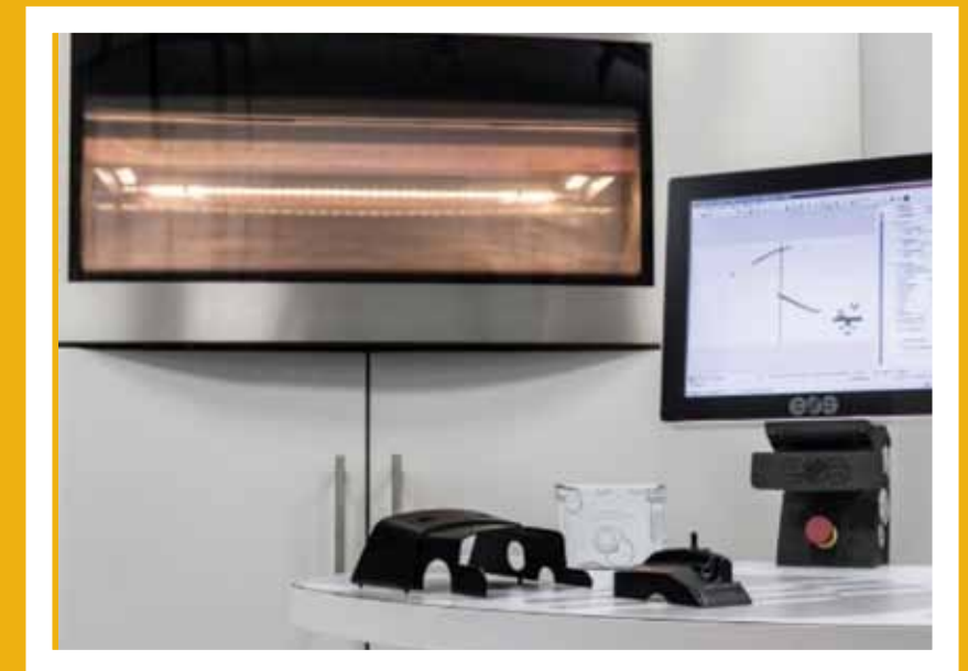
Mercedes-Benz Trucks already successfully produces 30 spare parts with the latest 3D SLS printing processes. Photo: Daimler
