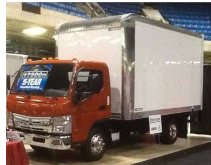
2014 MITSUBISHI FUSO CANTER FE125 Mitsubishi Engine, 4P10, 161 HP, Automatic Trans, 134" WB, 14 x 96" Van Body. Great Fuel Economy!
